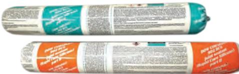
**DOWSIL™ 795** Silicone Building Sealant is a one-part, neutral-cure, architectural-grade sealant that easily extrudes in any weather and cures quickly at room temperature. This cold-applied, non-sagging silicone material cures to a medium- modulus silicone rubber upon exposure to atmospheric moisture. The cured sealant is durable and flexible enough to accommodate ±50 percent movement of original joint dimension when installed in a properly designed weather seal joint.
