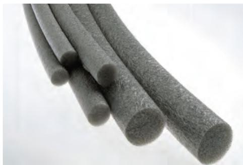
**Closed Cell Polyethylene** or **Open Cell Polyurethane** Foam Backer rod is used as compressible backup material in joints. It is inserted into a joint to control sealant depth creating a backstop that allows proper sealant curing, allows proper sealant wetting of the joint surfaces, insulate underside of sealant and acts as a bond breaker between the substrate and the sealant.
