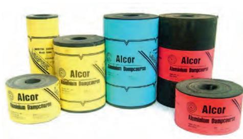
**Alcor** is a bitumen coated fully annealed 99% pure aluminium core Dampcourse supplied in various widths and thicknesses. The aluminium core is coated with bitumen on both sides and edges to prevent lateral corrosion.
