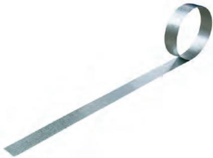
**TCS Galvanised Slipjoint** is supplied pre-greased with graphite grease sandwiched between an upper and lower sheet of 0.55 Galvanized hot dipped zinc coated commercial forming steel AS 1365. There are two basic variations available – standard flat or cavity bridge type.
