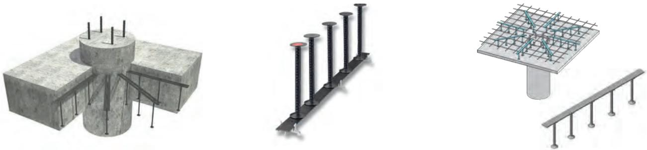
Shear Stud Punching Reinforcement Rails are a double-headed stud anchor reinforcement system, typically used for concrete deck-to-column connections. The system is designed to transfer the load further into the concrete deck, create a larger shear area around the column, and resist punching shear forces.
