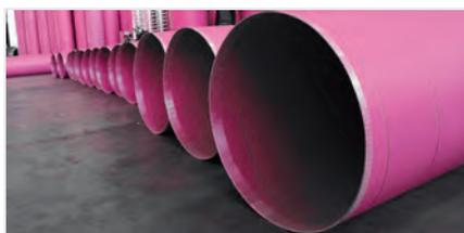
**Composite** tubing for concrete columns provide a light weight for ease of handling, waterproof for weather resistance, easy to cut to length, easy to strip alternative to conventional column forms. They are available in standard spiral tube or smooth lined to produce a smooth concrete finish.
