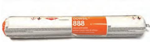
**DOWSIL™ 888** Silicone Joint Sealant and DOWSIL™ 890-SL Self-Levelling Silicone Joint Sealant are designed for use in roadway and airport joints calling for a tough sealant that can withstand excessive horizontal and vertical movement, has good weatherability and is easy to install with a short downtime and long service life one-part silicone. These sealants cure upon exposure to moisture in the air to form a permanently flexible, low- to ultralow-modulus, high-elongation silicone rubber seal.
