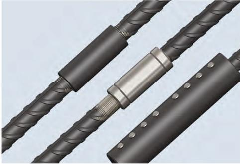
There are two main types of Reinforcement Bar Couplers – threaded bar type system or locking bolt/saddle type. The Threaded Bar type system consist of the coupler and the threaded bar to produce a full strength joint and best suited to large scale projects requiring a high volume of couplers. The end of each bar to be joined is threaded which screws into the threaded female coupling.
