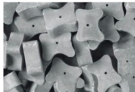
Bar chairs and spacers for concreting provide support for both reinforcing mesh and bar, ensuring that the correct cover of concrete over the reinforcement is achieved.
