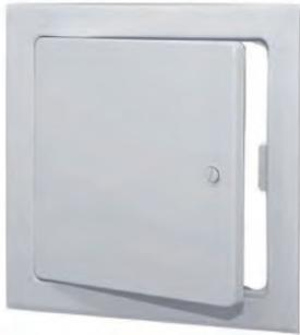
**Prefabricated Hinged Access Panels** are available in standard sizes non-rated, sound and fire rated constructed from mild steel, galvabond steel and stainless steel. Custom sizes are also available and can be manufactured to suit brickwork, Gyprock and/or tiled wall.
