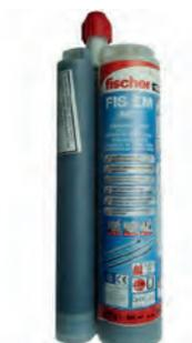
**Fischer FIS EM** is a powerful epoxy resin mortar injection system. When combined with a threaded rod, is suitable for pre-positioned and push-through installation. Resin and hardener are stored in two separate chambers and are not mixed and activated until extrusion through the injection capsule in the static mixer. The mortar is injected bubble-free from the drill hole base.
