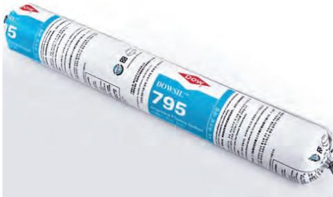
**DOWSIL™ 795** Silicone Building Sealant is a one-part, neutral-cure, architectural-grade sealant that easily extrudes in any weather and cures quickly at room temperature. This cold-applied, non-sagging silicone material cures to a medium- modulus silicone rubber upon exposure to atmospheric moisture. The cured sealant is durable and flexible enough to accommodate  $\pm 50$  percent movement of original joint dimension when installed in a properly designed weather seal joint.
