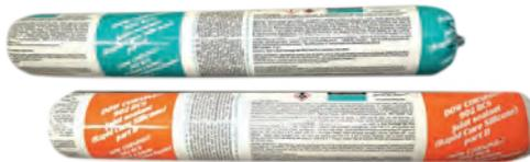
**DOWSIL™ 902** RCS Joint Sealant is a rapid-cure, self-levelling, two-part silicone rubber sealant designed to seal expansion joints primarily intended for use in expansion joints found on bridges that vary in width from 25 to 76 mm at the time of sealing.
