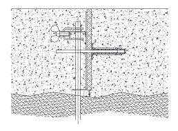
The Stiff foam can be left in-situ or later mechanically removed and sealant installed if desired. The pre-cut foam profile is 10mm above the metal top edge.
