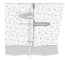
The plastic capping is concrete grey in colour, UV stable and easily installed along the joint length. Capping can be left in-situ or later removed to provide a void for installation of an elastomeric sealant if desired.
