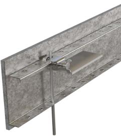
EXA-Joint® consists of the plain joint assembly which includes plate dowels welded in position, rigid plastic dowel sleeves, metal stakes and adjustment clamps.
