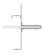
With the addition of profile cut stiff foam sheets, the EXA-Joint<sup>®</sup> is used as an expansion joint which allows for thermal expansion of the slab.
