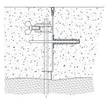
The plastic capping is concrete grey in colour, UV stable and easily installed along the joint length. Capping can be left in-situ or later removed to provide a void for installation of an elastomeric sealant if desired.
