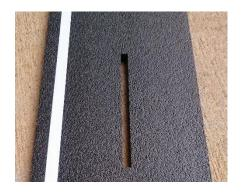
Galvanised Plate Dowels & Sleeves provide superior load transfer across the joint (refer to Dowel Capacity Comparison Chart). Each dowel is welded in position and fitted with rigid plastic dowel sleeves - no need for on-site assembly of dowels and sleeves
